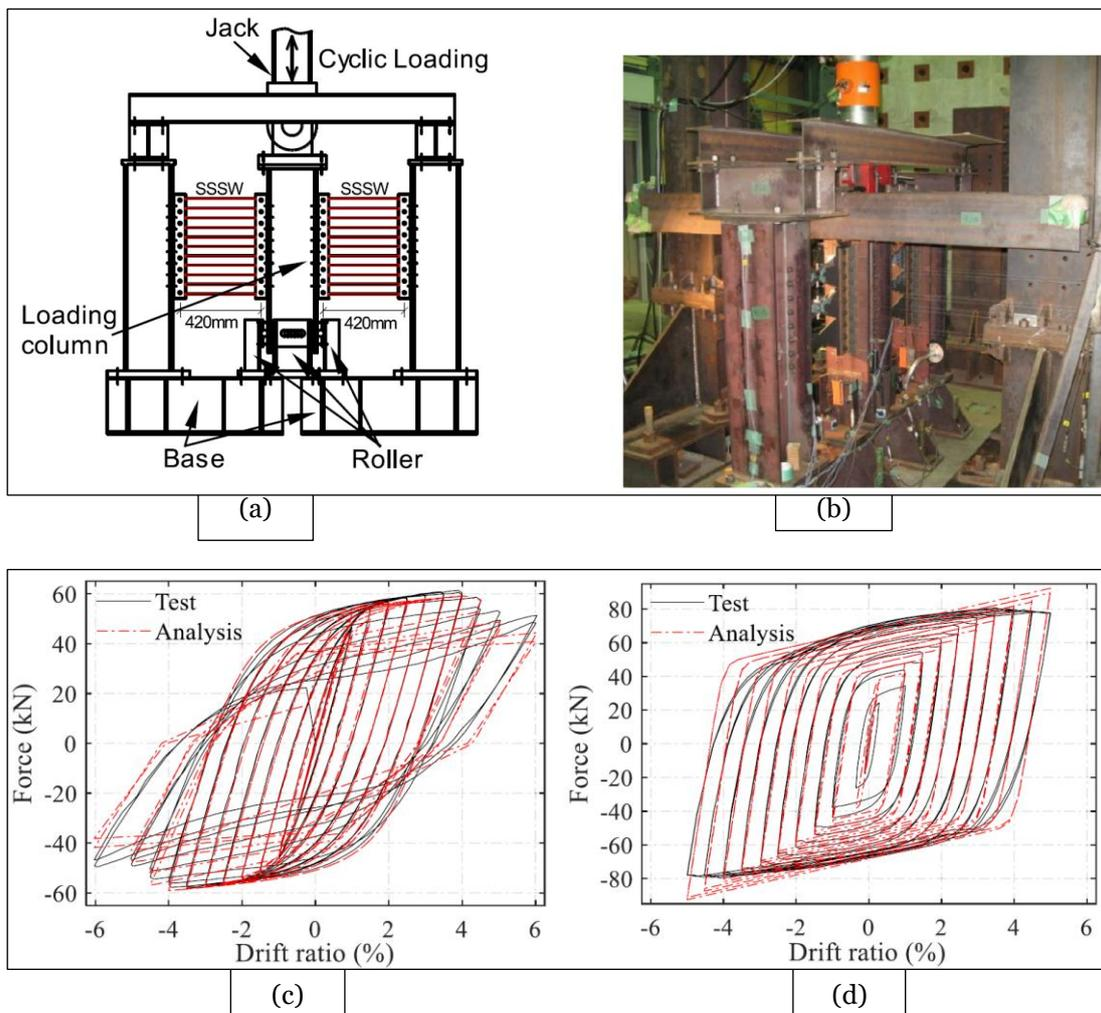
**Fig. 10: (a) Illustration of test setup. (b) Test setup. (c) Test and simulation results for SSSW made of mild carbon steel. (d) Experimental and numerical results for SSSW made of low yield steel [64]**
