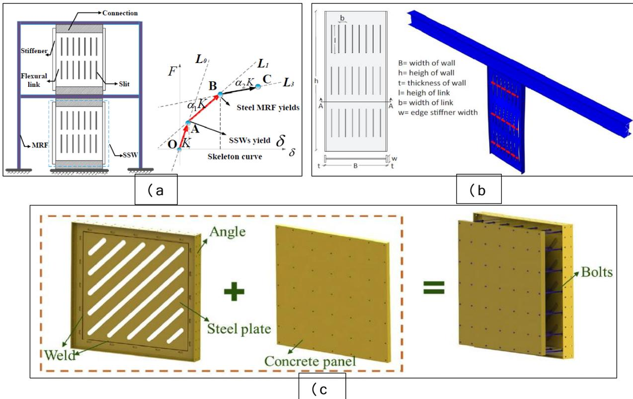
Fig. 9 : (a) Multi-yielding stages of a steel MRF outfitted with slit steel wall [59]. (b) Slit panel geometry with a vertical slit [60]. (c) SPSW configuration with inclined slots [61]
