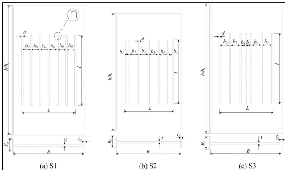
Fig. 5: Slit walls with non-uniform spacing [28]
