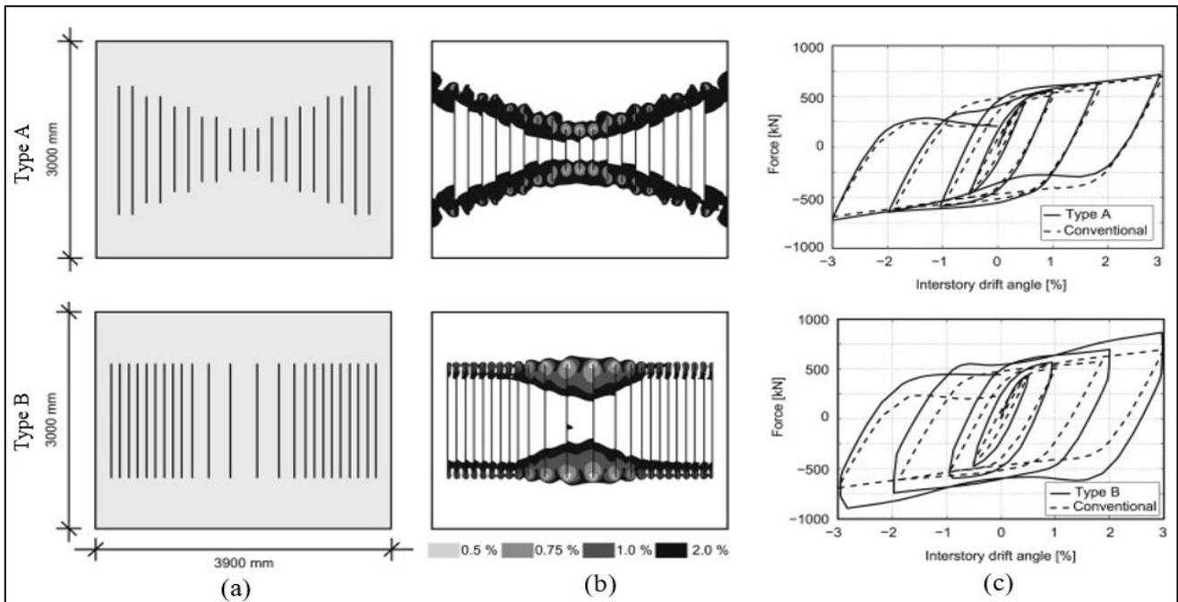
**Fig. 3: Modified slit walls [48]: (a) Slit types. (b) Stress distribution. (c) Hysteretic behavior**
