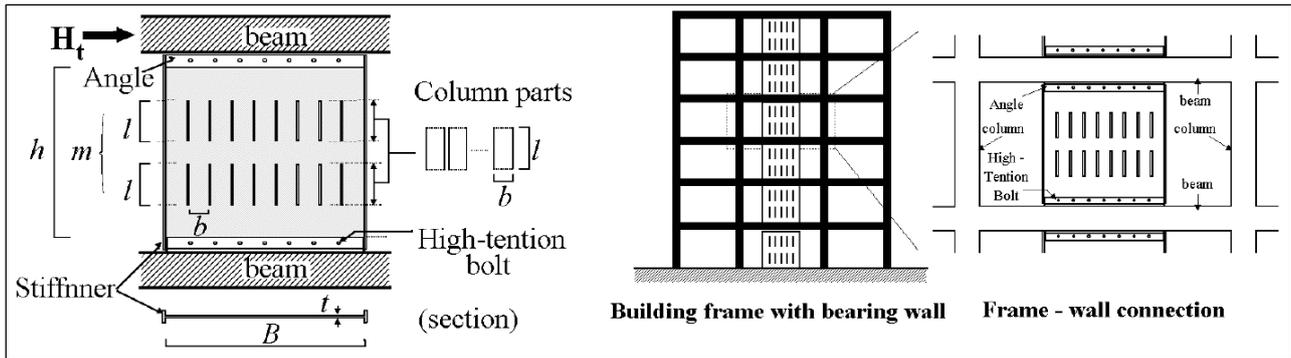
**Fig. 2: Slit steel walls [46]**
