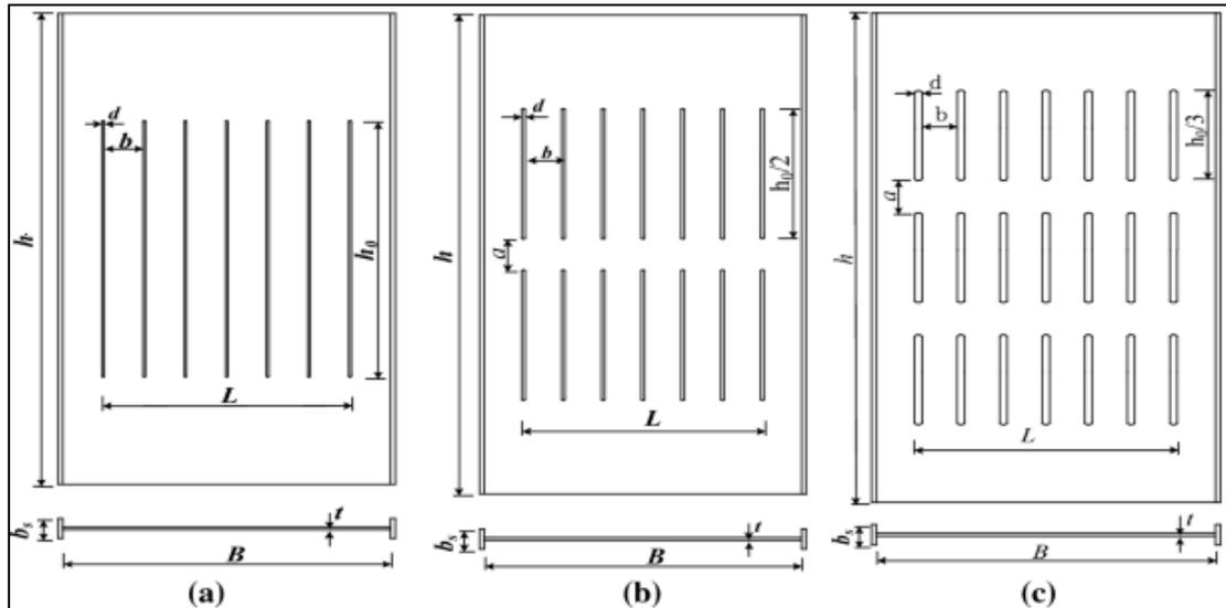
Fig. 6: Patterns of steel walls with multilayer slits [55]: (a) Single-layer slit. (b) Two rows of links. (c) Three rows of links
