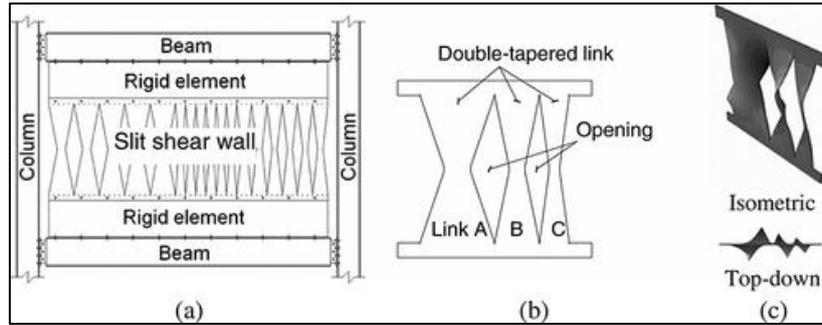
Fig. 4: Slit wall with double-tapered links [53]
