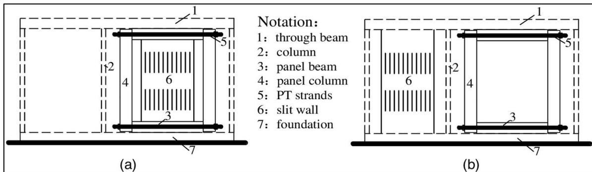
Fig. 8: An example of a SCMP-SW elevation arrangement [57]: (a) Assembled type. (b) Separated type
