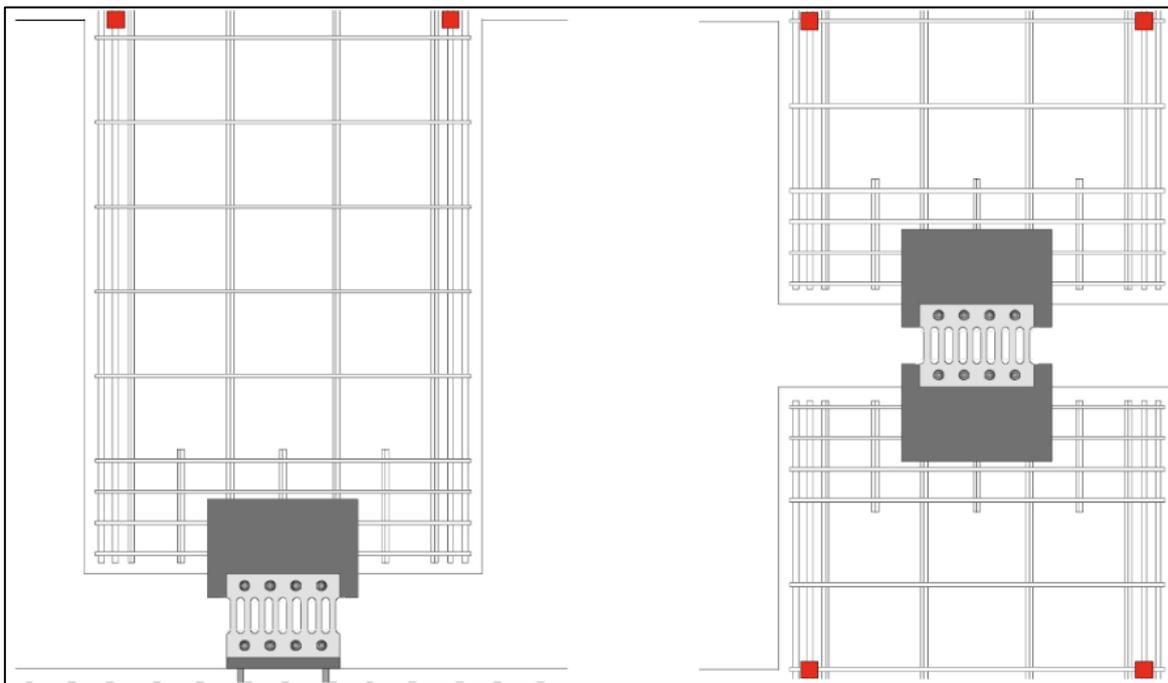
**Fig. 11: Using Slit dampers in Lightly reinforced concrete (LRC) walls**
