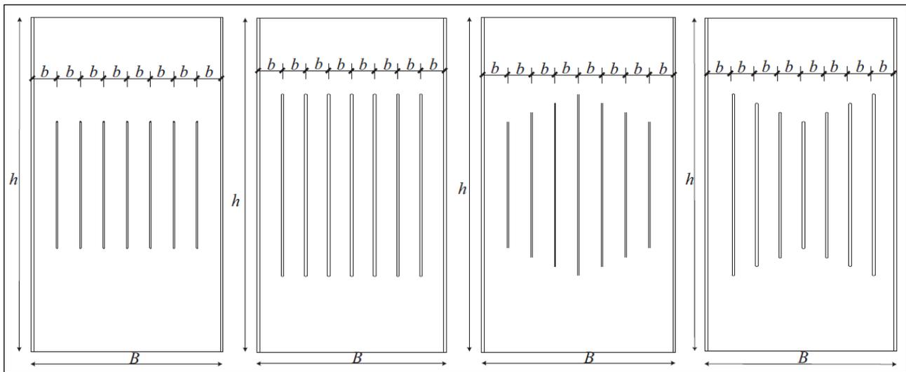
Fig. 7: Patterns of steel walls with unequal length slits [56].
