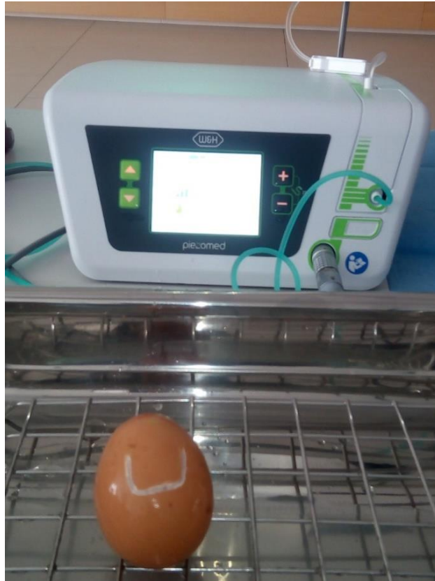
Figure 4: Section performed on the eggshell by ultrasound microvibration emitted by the piezoelectric device shown in the photo
