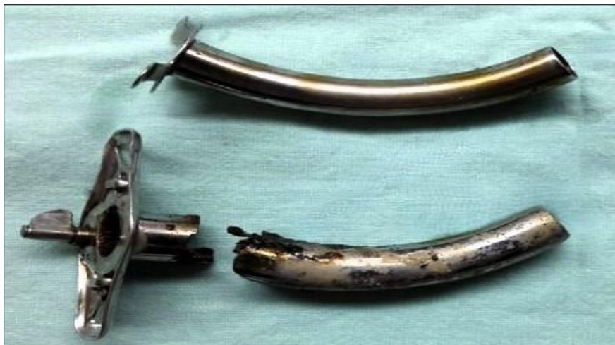
Figure 2: Fractured tracheostomy tube expelled by the patient during a coughing effort, compared to an intact Krishaber tracheostomy tube.
