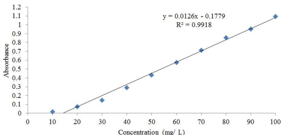
Fig-1: Glucose standard curve for EPS yield determination
