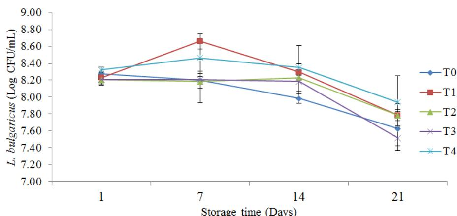
**Fig-2: Interaction between addition level of Canna starch and CMC on *L. bulgaricus* viability during storage ( $p < 0.05$ ). Error bars represent standard deviation**
