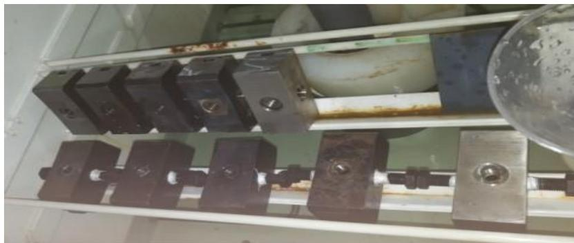
**Figure 8: Clutch air spring gas line pins before salt spray test**
