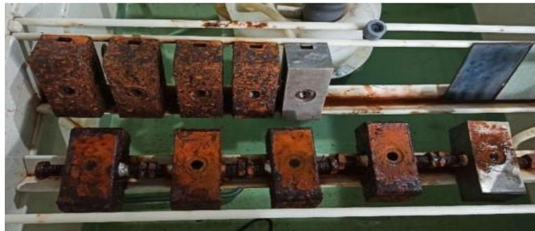
**Figure 12: Clutch air spring gas line plug after eighteen days of salt spray test**
