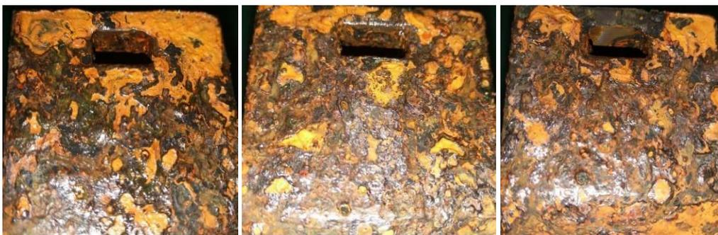
**Figure 13: Corrosion of three sets of test pieces (after cleaning)**
