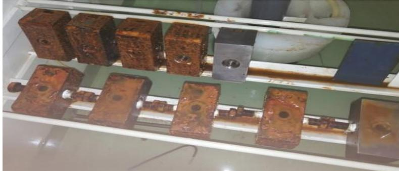
**Figure 10: Clutch air spring gas line plug after four days of salt spray test**
