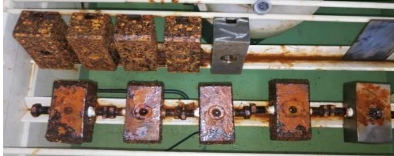
**Figure 11: Clutch air spring gas line spigot status after thirteen days of fog test**
