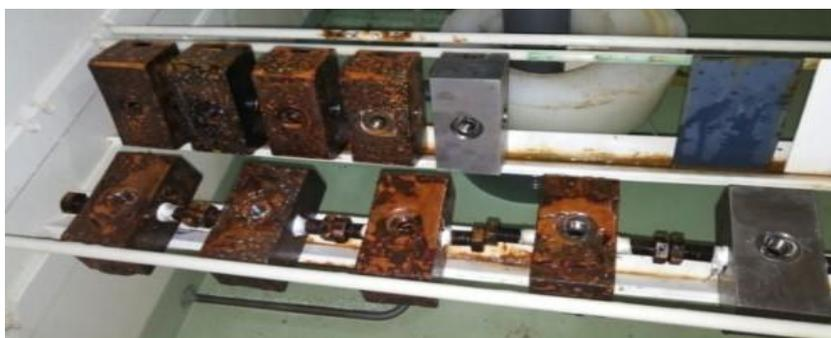
**Figure 9: Clutch air spring air circuit after one day of salt spray test**
