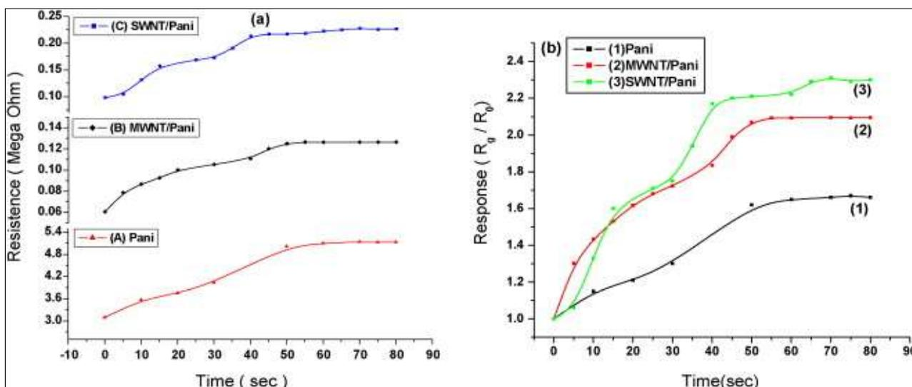
**Figure 4: (a) Recorded changes in resistance of the composite material upon exposure to 2% H<sub>2</sub>; (b) Sensor response profile of the composite at a hydrogen concentration of 2%**
