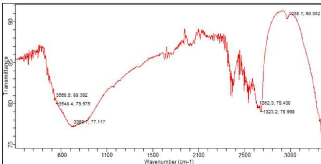
**Figure 1: FTIR Spectrum for Nickel Oxide Nanoparticles**
