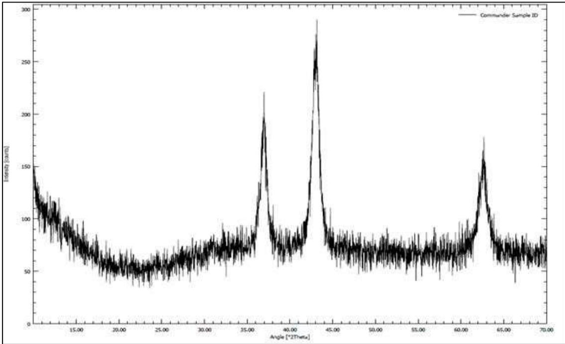
**Figure 3: X-ray Diffraction image Nickel Oxide Nanoparticles**
