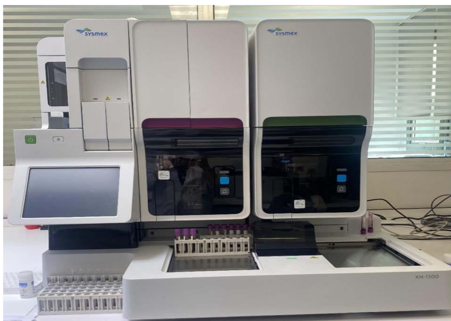
Figure 1: Sysmex XN-1500 machine used to perform CBC in the laboratory
