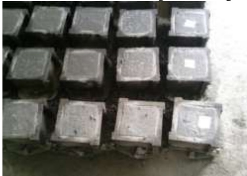
Figure 1: Concrete Cubes Specimens
