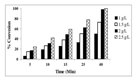
Figure 5. Effect of Catalyst quantity
