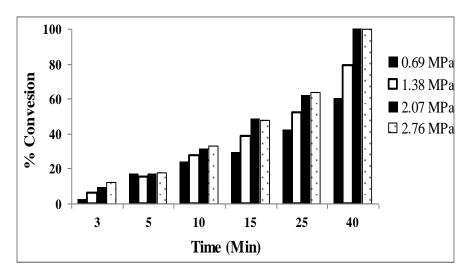
Figure 4. Effect of Hydrogen partial pressure
