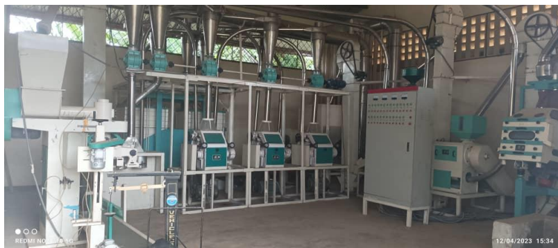
Picture 4: CUSABU milling machine with capacity of grinding 30 tons per day, Musigati, Bubanza. Source: Research on field
