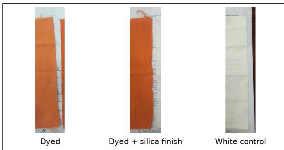
Figure 2: Fabric conditions used in the broader test programme: white control and orange dyed specimens, including the dyed silica-finished condition (laboratory record)
