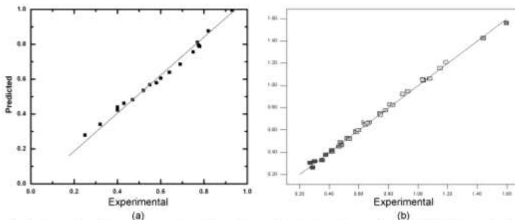
Fig. 9: Comparison between the experimental and the predicted values of dimensionless height of top packed bed formation by (a) dimensional analysis and (b) statistical analysis
