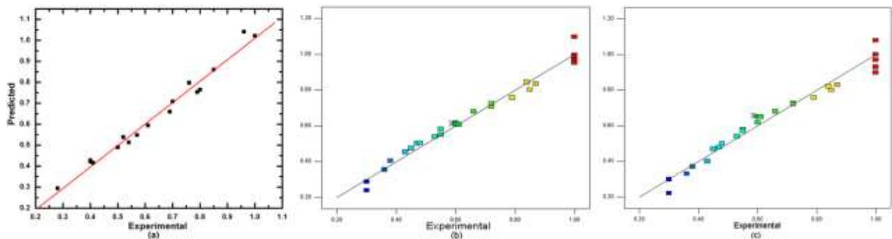
Fig. 5: Comparison between the experimental and the predicted values of dimensionless height of top packed bed formation by (a) dimensional analysis, (b) statistical analysis (Quadratic) and (c) statistical analysis (Linear)
