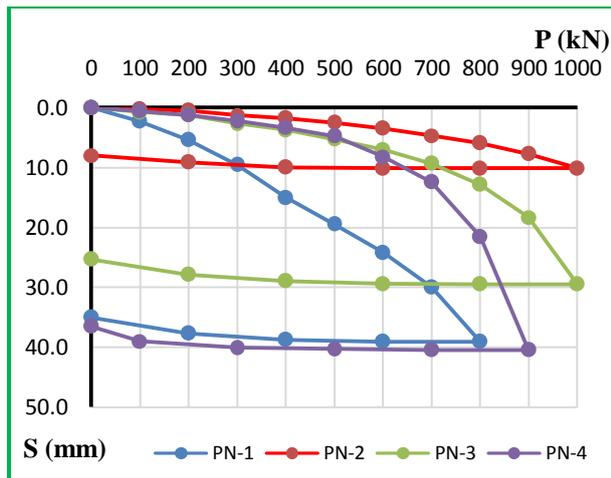
Fig.7: Load-settlement of four tested piles
