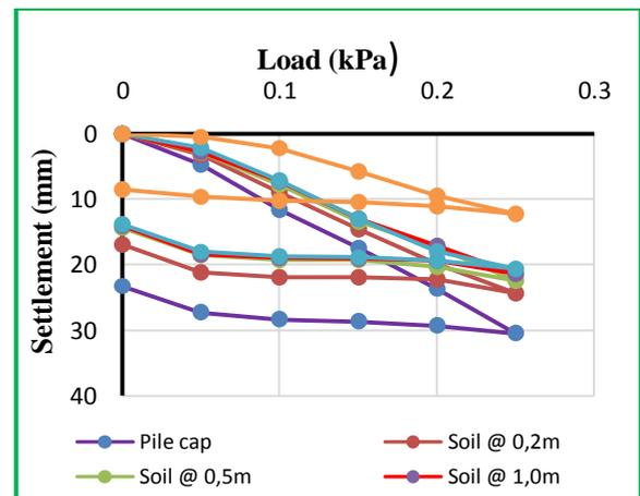
**Fig.8: Settlement of soils under cap of PN-4**
