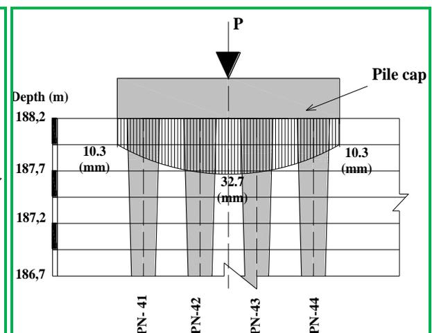
Fig.12: Horizontal Settlement of pile PN-4
