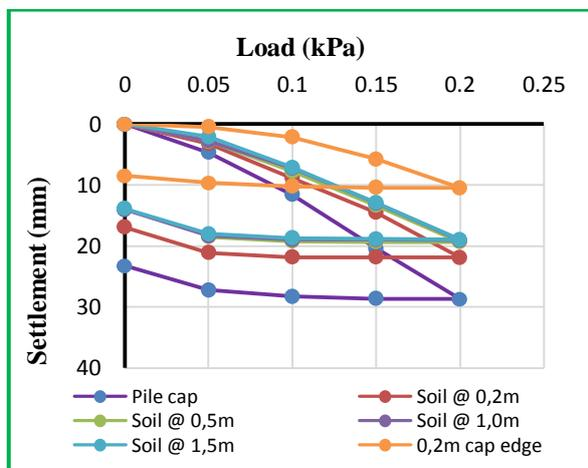
**Fig.5: Settlement of soils under cap of PN-1**
