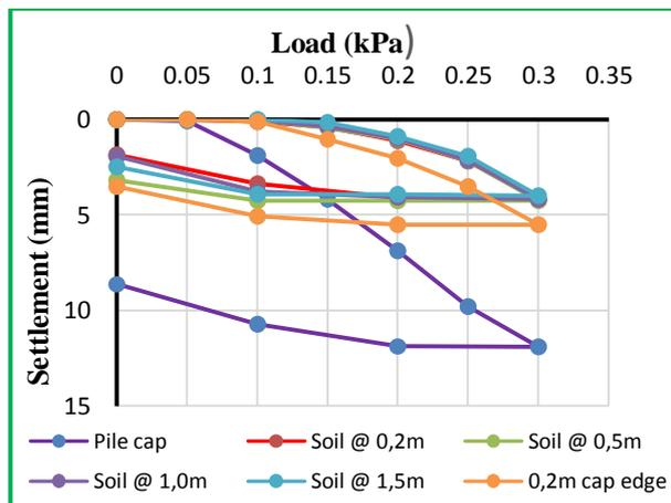
**Fig.7: Settlement of soils under cap of PN-3**
