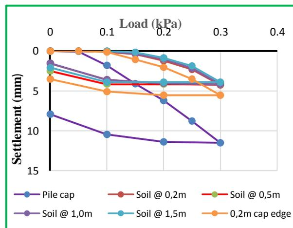
**Fig.6: Settlement of soils under cap of PN-2**
