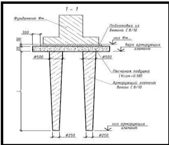
**Fig.3:Tapered Piles section on the field**
