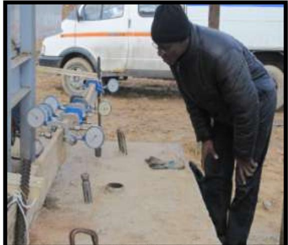
**Fig.4: Taking Settlement Reading on Dial gauges**
