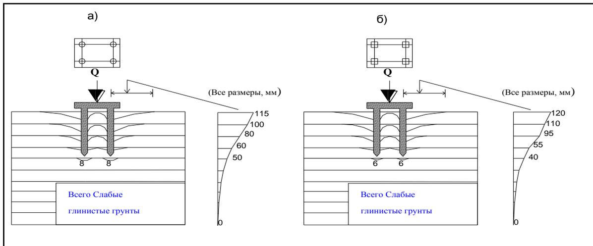
**Fig.7: Deformation of 2x2-pile group for Case-4 soil condition: (a) - cylindrical shaped piles (б) tapered conical section.**
