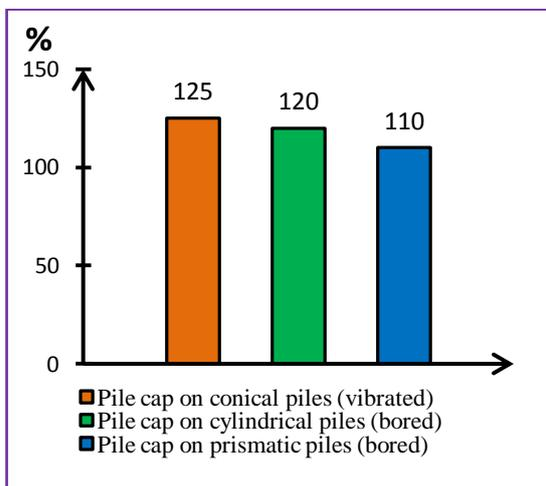
Fig.15: B/Capacity of pile & pile cap - case 1
