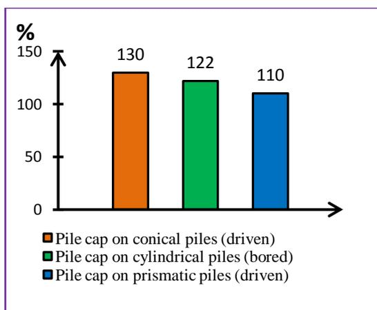
Fig.17: B/Capacity of pile & pile cap - case 5
