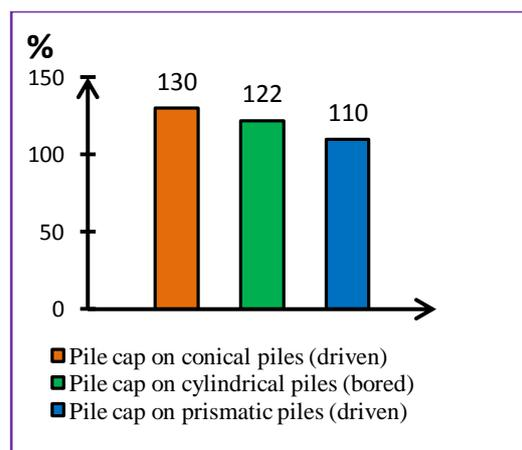
Fig.18: B/Capacity of pile & pile cap - case 7
