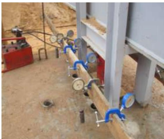
Fig.5: Dial gauges for Settlement Reading
