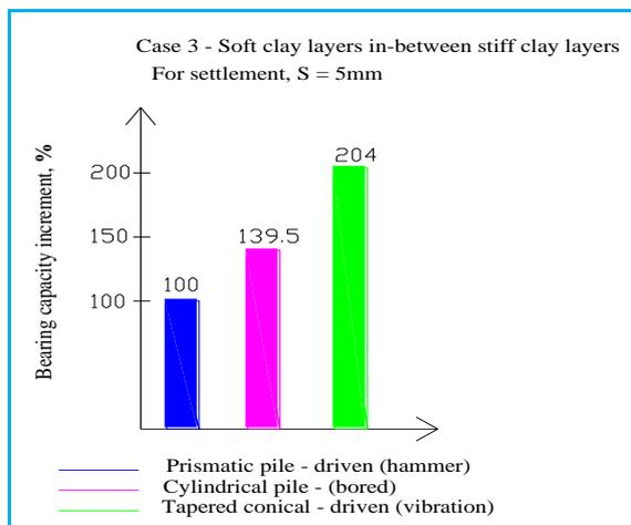
Fig.10: Bearing capacity of piles - case 3
