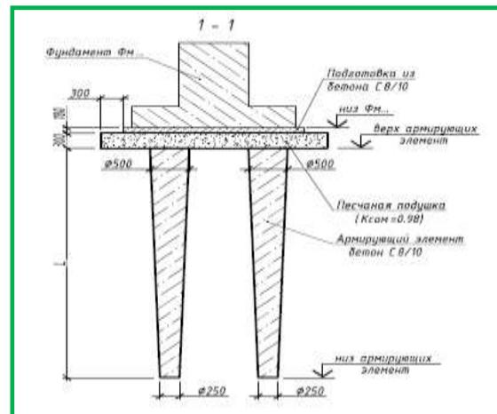
Fig.6: Section of conical shaped pile
