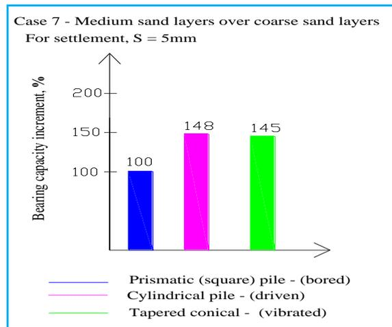
Fig.14: Bearing capacity of piles - case 7
