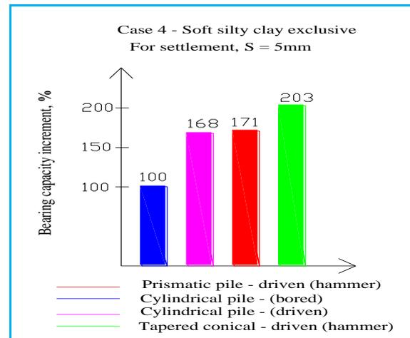
Fig.11: Bearing capacity of piles - case 4
