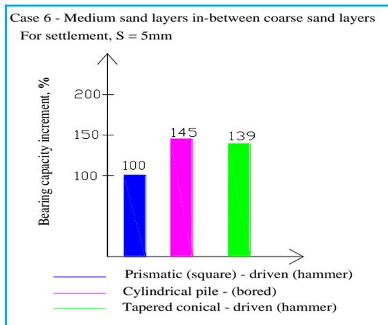
Fig.13: Bearing capacity of piles - case 6
