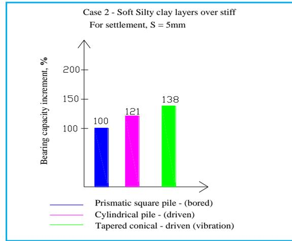
Fig.9: Bearing capacity of piles - case 2
