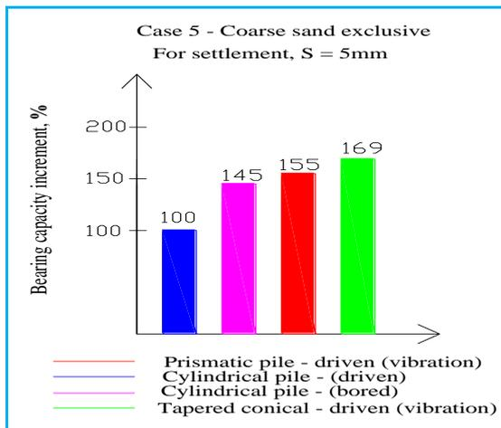
Fig.12: Bearing capacity of piles - case 5
