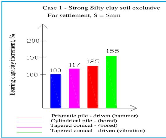
Fig.8: Bearing capacity of piles - case 1
