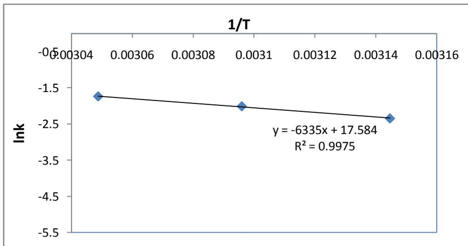
Fig- 6: Dependence of drying rate constant on temperature
