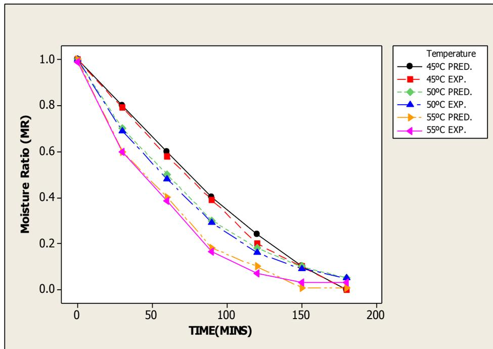
Fig-5: Experimental and predicted moisture ratio by the Henderson and Pabis model versus drying time for leather with 30% dextrinized sweetpotato
