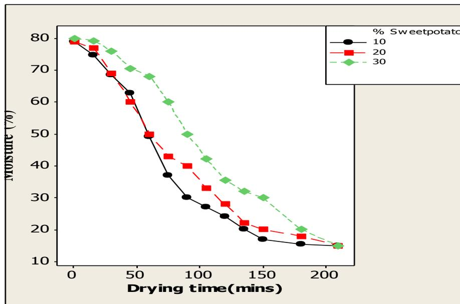
Fig-3: Effect of dextrinized sweetpotato on drying rate of leathers
