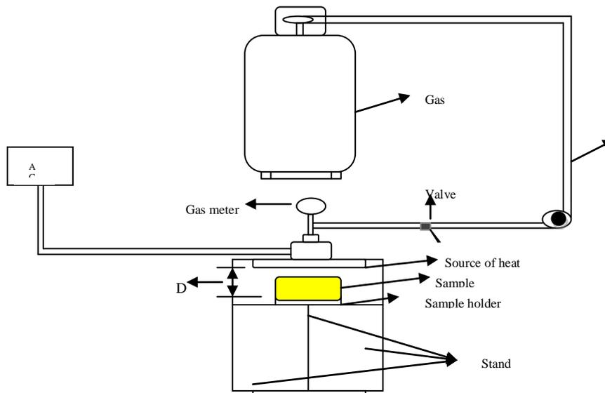
**Fig-1: Schematic diagram of the catalytic infra-red dryer**
