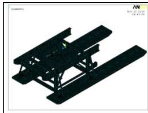
Fig-13: The meshed model of the substructure
