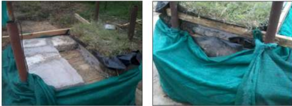
Fig. 1: Experimental setup: RCC slabs with and without grass covering (left); polyethylene layer and green net as walls for insulation (right)
