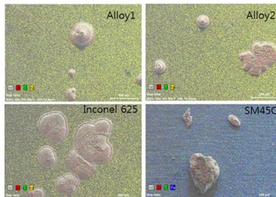
**Fig. 3: Mapping (EDS) configuration of samples with Zn oxide**
