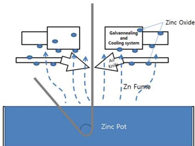
Fig. 1: Schematic diagram for hot dip galvanizing equipment
