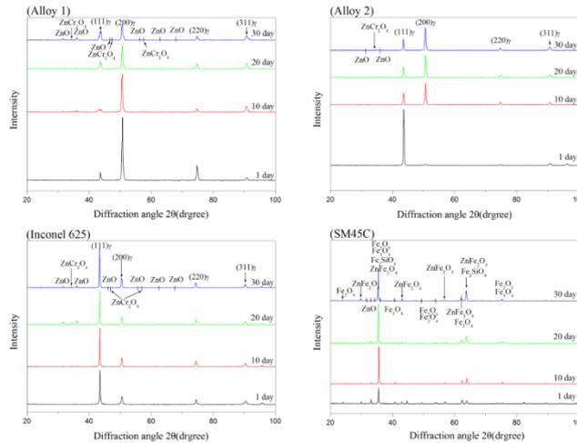
**Fig. 4: X-ray peak after corrosion of each material in the environment with high temperature and Zn fume**
