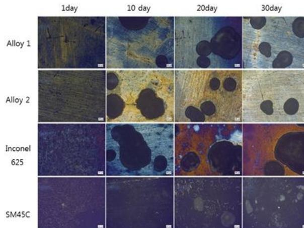
**Fig. 2: Photos of optical microscope after the oxidation experiment with Zn fume**
