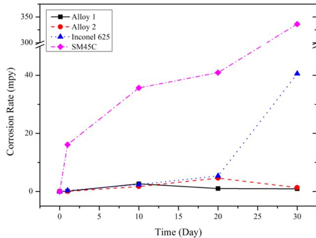
**Fig. 6: Corrosion Rate(mils per year)**
