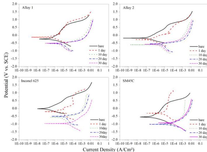
**Fig. 5: Potentiodynamic polarization graph of each material**
