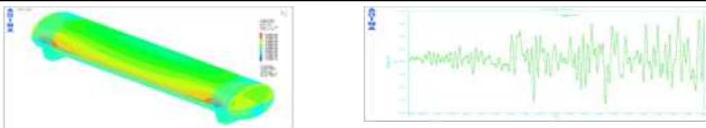
Fig. 6 the horizontal tank axial stress nephogram in Taft wave
