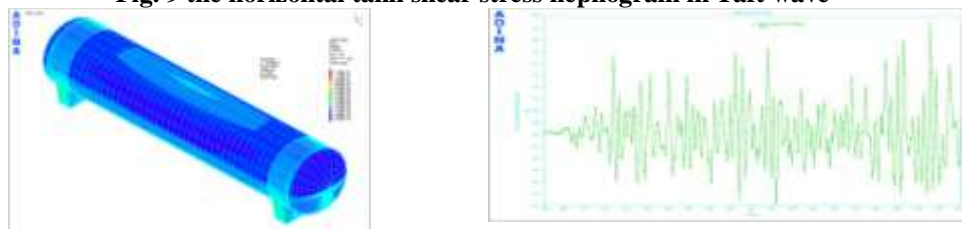
Fig. 10 the horizontal tank shear stress nephogram in artificial wave
