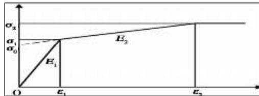
Fig-1: Simplified diagram of three line model of stress-strain relationship
