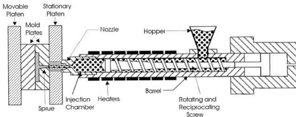
**Fig-1: Schematic diagram of an injection mould process**
