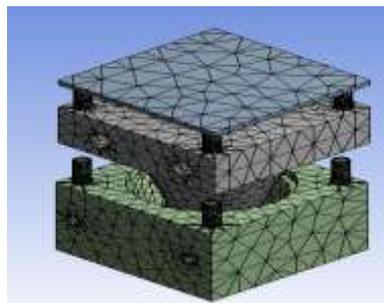
Fig-4: Fine size meshing of the isometric view of the cavity and core mould
