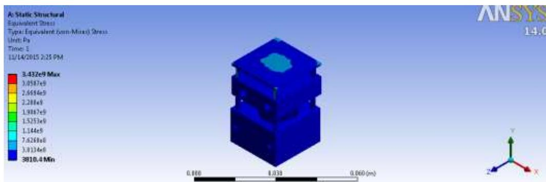
Fig-8: equivalent Von mises of the static analysis of the treated injection mould
