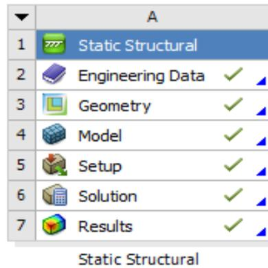
Fig-3: flow diagram of the structural analysis of the Ansys workbench 14.0
