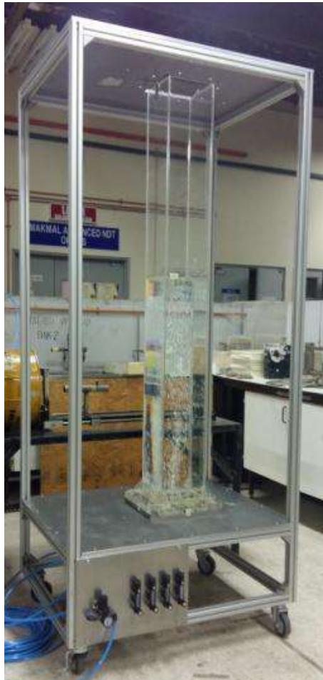
Fig-8: The final prototype reactor
