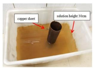
Fig-4: Diagram of electrochemical corrosion test apparatus
