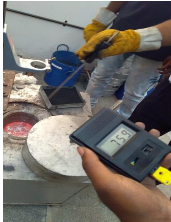
Fig-1: Al-3Mg/ SiC/Gr. in liquefied pouring temperature of 760 ^{\circ}\text{C} .
