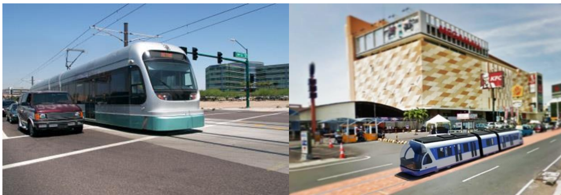
Figure 1: The LRT rail is the same level with the highway (Barrett et al. , 2019)
