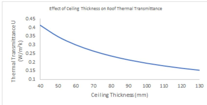
**Fig-7: Effect of Ceiling Layer Thickness on Roof Thermal Transmittance**
