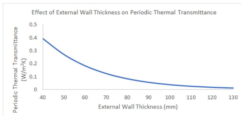
**Fig-13: Effect of Wall Layer Thickness on Wall Periodic Thermal Transmittance**
