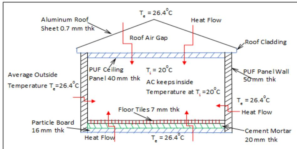
Fig-3: A sketch showing the construction details and heat flow
