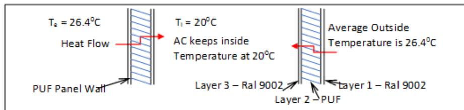
Fig-4: A sketch showing the wall thermal layers
