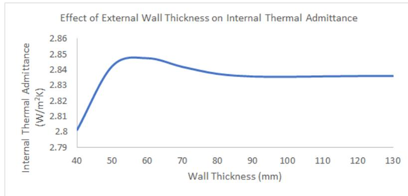
**Fig-14: Effect of Wall Layer Thickness on Wall Thermal Admittance**
