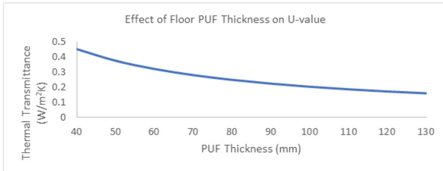
**Fig-16: Effect of Floor PUF Layer Thickness on Floor Thermal Transmittance**
