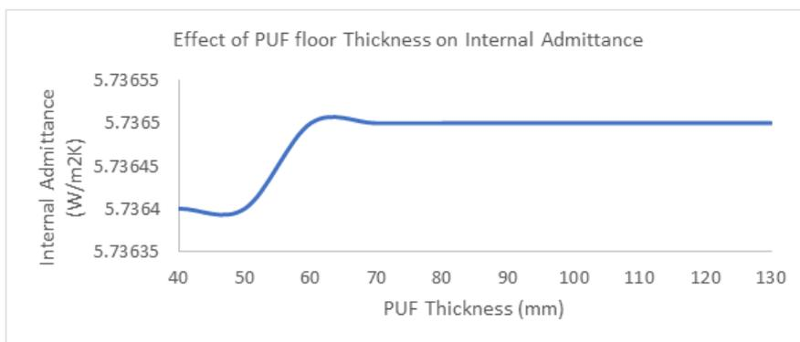
**Fig-18: Effect of Floor PUF Layer Thickness on Floor Thermal Admittance**
