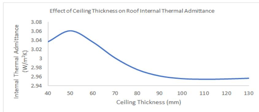
**Fig-10: Effect of Ceiling Layer Thickness on Roof Thermal Admittance**
