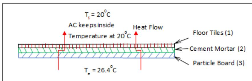
Fig-6: A sketch showing the floor thermal layers
