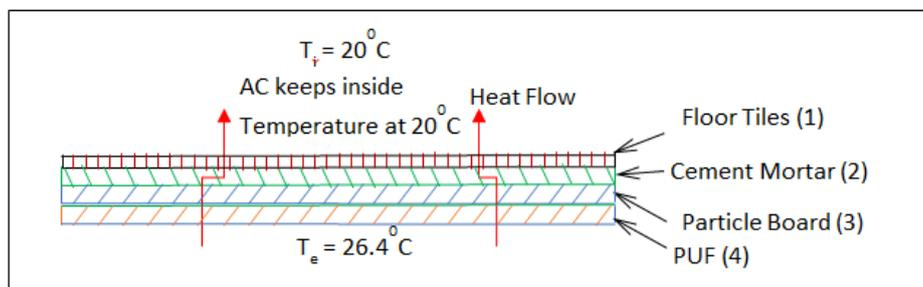
**Fig-15: A Sketch of modified Floor Construction and thermal layers**
