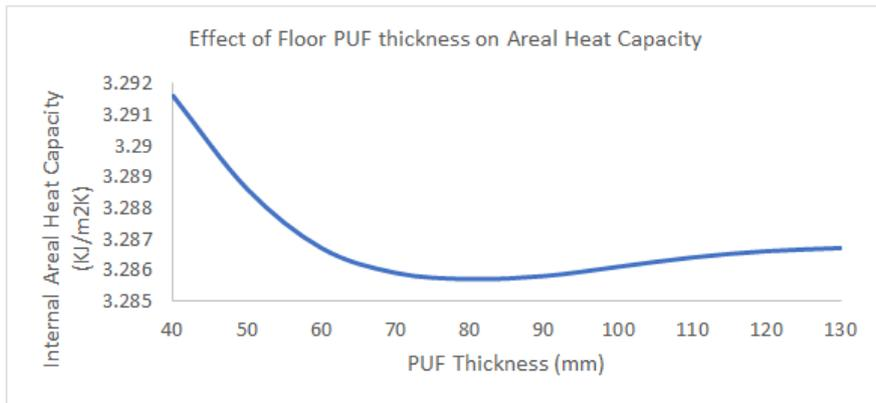
**Fig-17: Effect of Floor PUF Layer Thickness on Floor Areal Heat Capacity**
