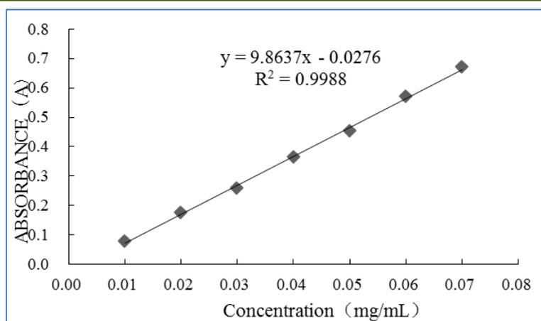
**Fig-1: Glucose standard curve**
