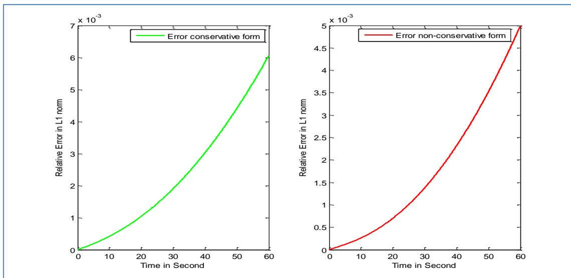
Fig-6: Comparison of relative errors between conservative and non-conservative form
