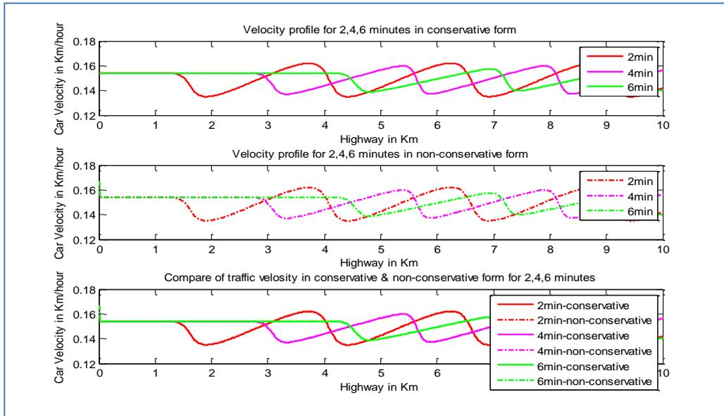
**Fig-3(b)(i): Velocity profile conservative and non-conservative form of 2, 4, 6 minutes (linear) in a 10 km highway**
