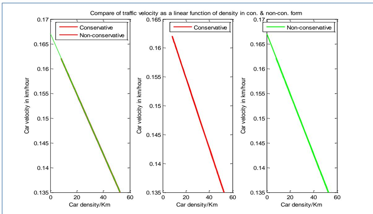
**Fig-4(i): Traffic velocity as a function of density (linear case) conservative and non-conservative form**
