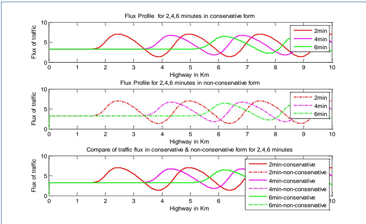
**Fig-3(c)(ii): Flux profile conservative and non-conservative form of 2, 4, 6 minutes (non-linear) in a 10 km highway**
