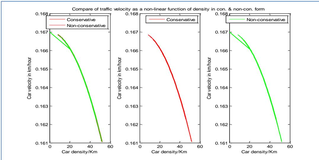
**Fig-4(ii): Traffic velocity as a function of density (non-linear case) conservative and non-conservative form**
