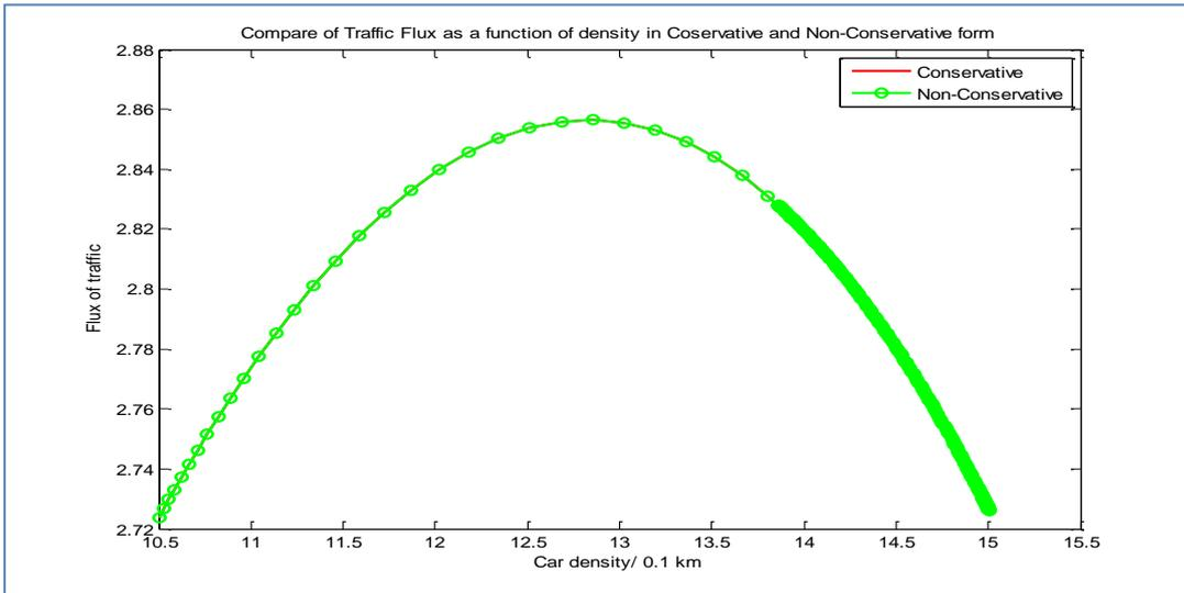
**Fig-5(i): Traffic Flux as a function of density (linear case) conservative and non-conservative form**
