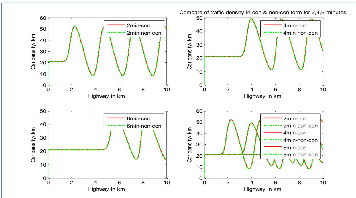
**Fig-3(a): Density profile conservative and non-conservative form of 2, 4, 6 minutes in a 10 km highway**
