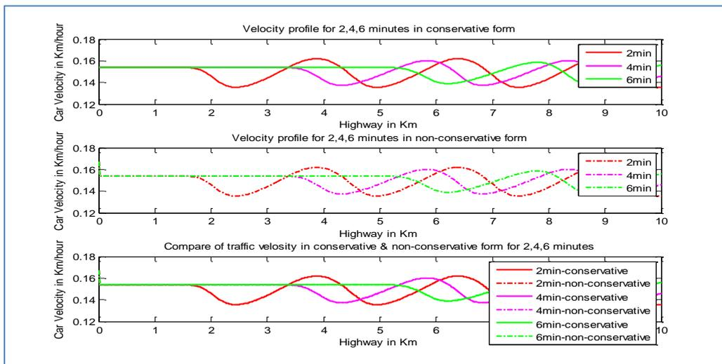
**Fig-3(b)(ii): Velocity profile conservative and non-conservative form of 2, 4, 6 minutes (non-linear) in a 10 km highway**
