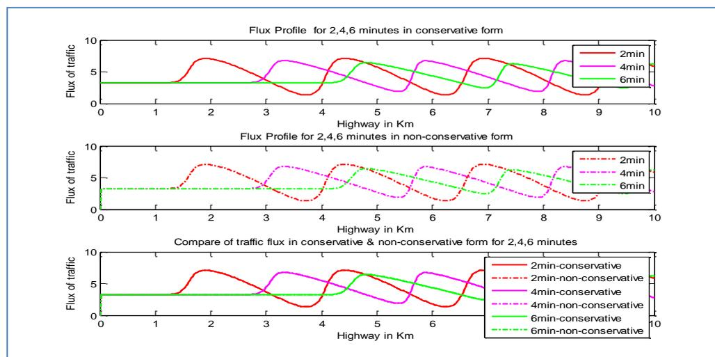
**Fig-3(c)(i): Flux profile conservative and non-conservative form of 2, 4, 6 minutes (linear) in a 10 km highway**
