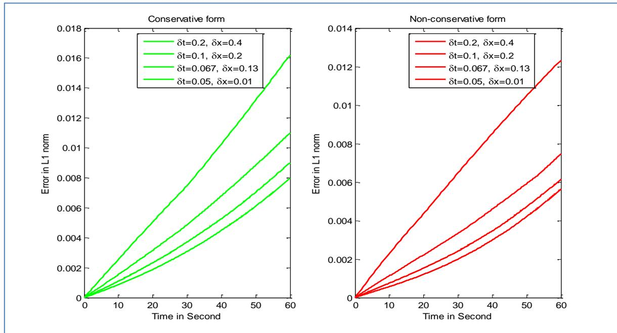
**Fig-7: Comparison of convergence errors between conservative and non-conservative form**
