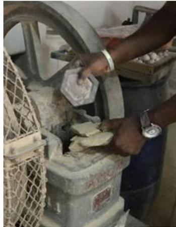
**Fig-3: Crushing the clay**
