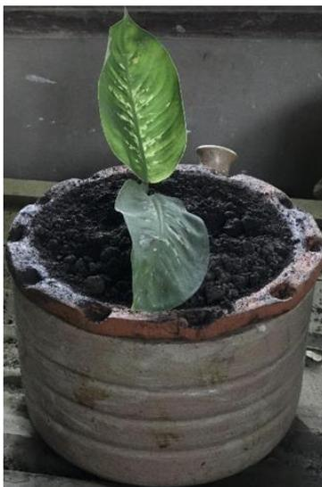
**Fig-17: Planter 2 with the vitrified body as the reservoir (Body B)**
