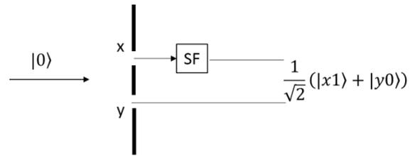
**Figure 1: Generation of hybrid entangled state. SF represents spin flipper**
