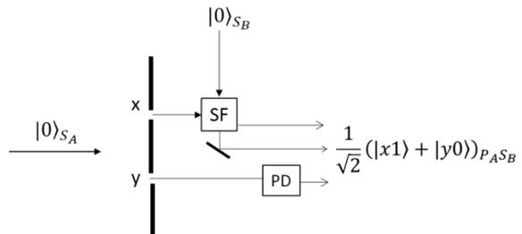
**Figure 2: Generation of hyper entangled state. SF and PD represent spin flipper and path detector respectively. SF is activated only when particle A incident on it and then it flips the spin of particle B. Here, PA and SB stand for path and spin of particles A and B respectively**
