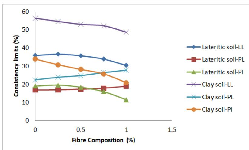
**Figure 3: Plot of consistency limits versus bagasse fibre in cement stabilized soil**
