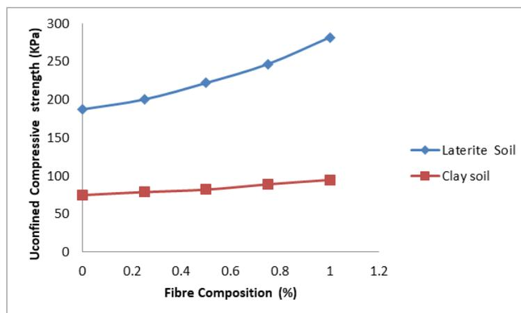
Figure 5: Plot of unconfined compressive strength versus bagasse fibre in cement stabilized soil
