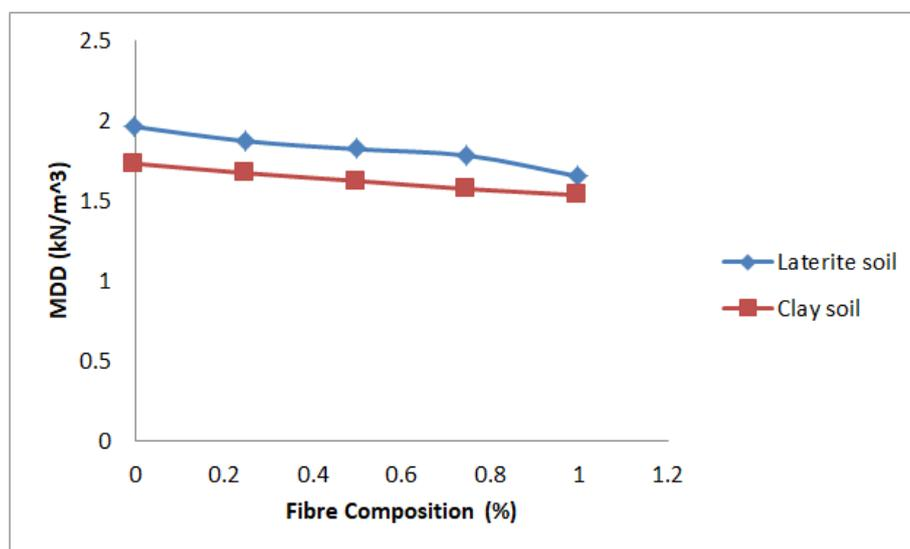
**Figure 1: Plot of MDD versus bagasse fibre in cement stabilized soil**
