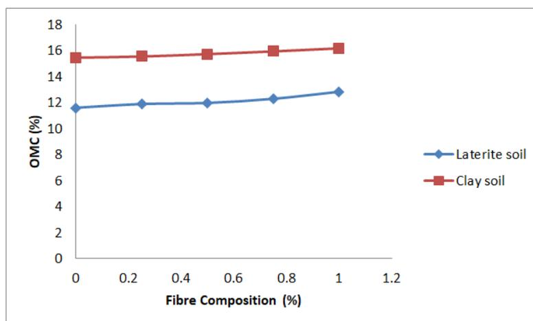
**Figure 2: Plot of OMC versus bagasse fibre in cement stabilized soil**
