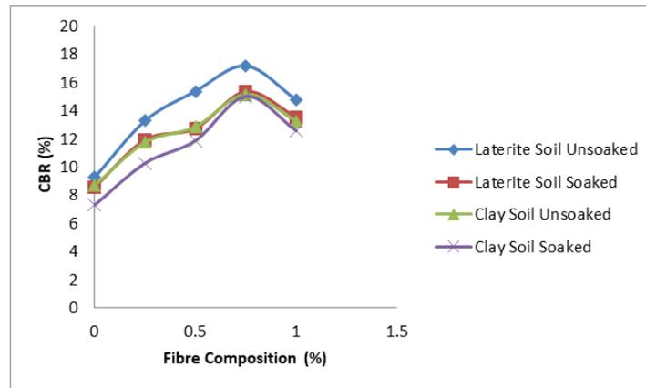
Figure 4: Plot of CBR versus bagasse fibre in cement stabilized soil
