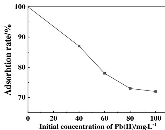
Fig 2: Effect of initial concentration of Pb(II) on adsorption rate
