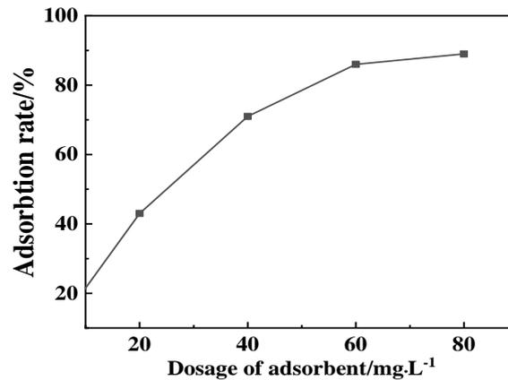
Fig 1: Effect of adsorbent dosage on adsorption rate of Pb(II)
