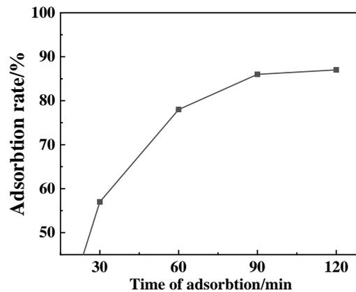
**Fig 3: Effect of adsorption time on the adsorption of Pb(II)**
