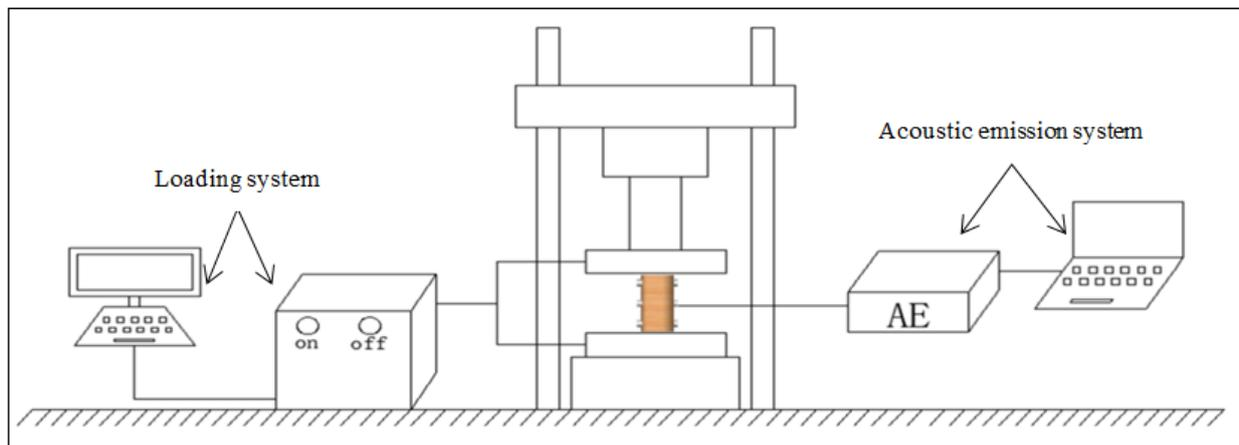
**Fig 1: Loading schematic**
