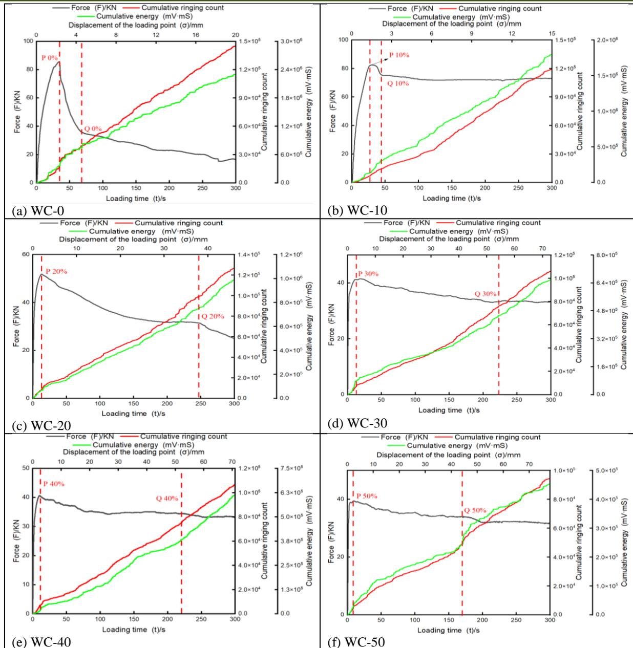
**Fig 9: Acoustic emission cumulative ringing count and cumulative energy**
