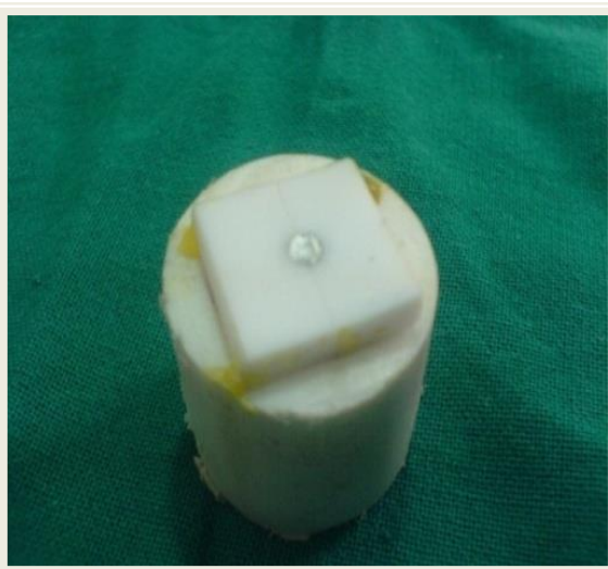
(Fig. 7) The Sample after Compaction of the Amalgam
