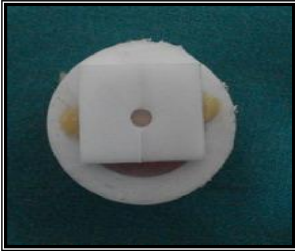
(Fig.3) Applying the Teflon Mold to the Sample Surface
