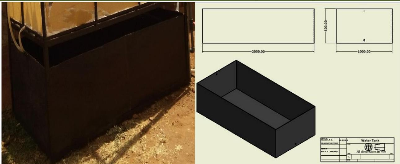
**Figure 3: Designed Water tank (reservoir)**
