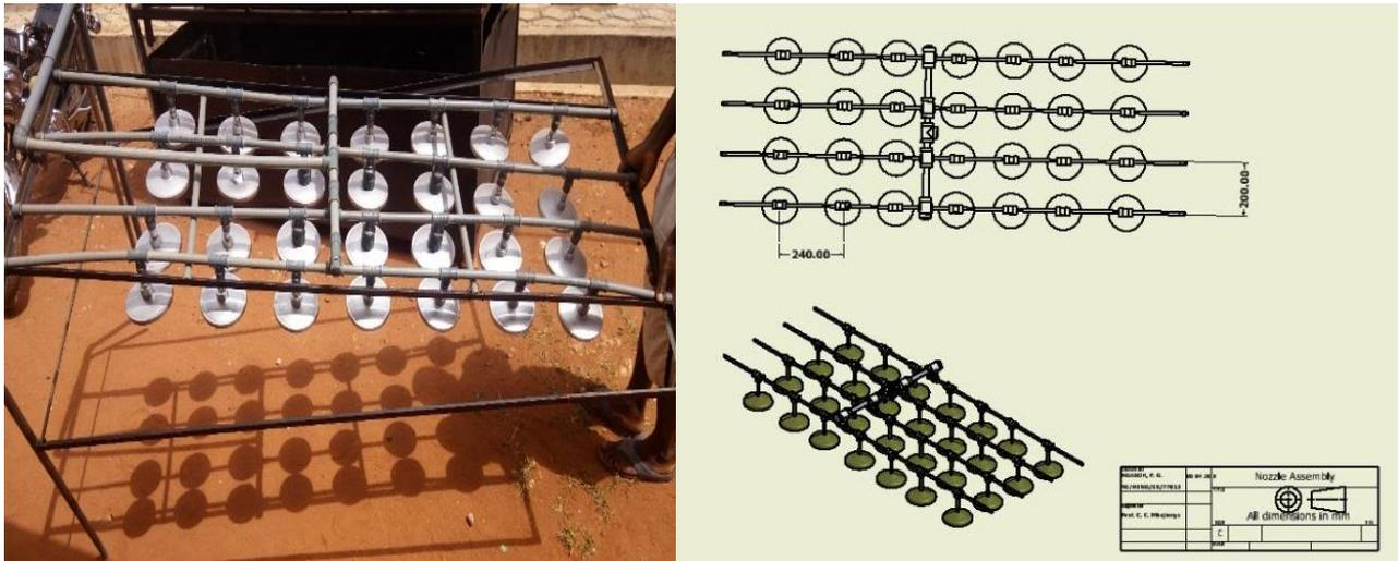
Figure 1: Nozzles arrangement
