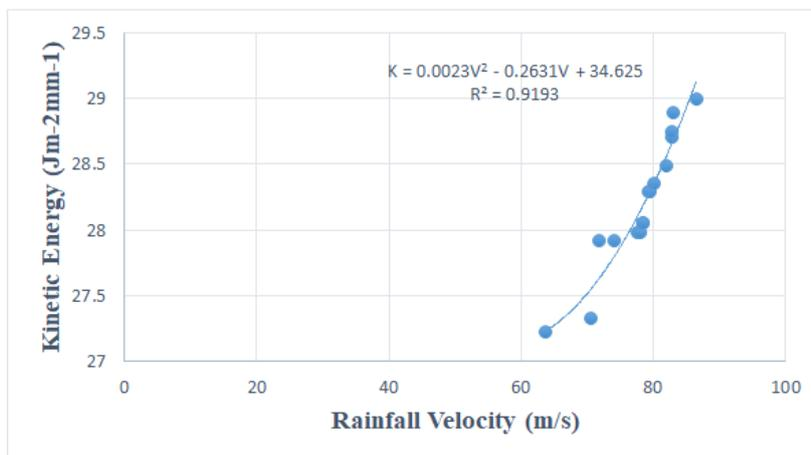
Figure 10: Graph showing the relationship between Kinetic energy and drop velocity
