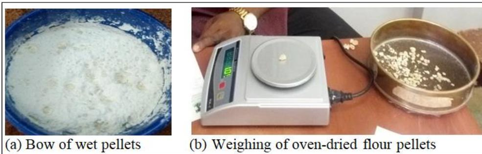
**(a) Bow of wet pellets (b) Weighing of oven-dried flour pellets**
