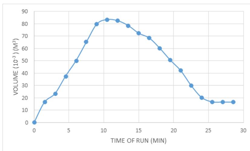
Figure 11: Hydrograph of runoff discharge for 7 minutes simulated rainfall
