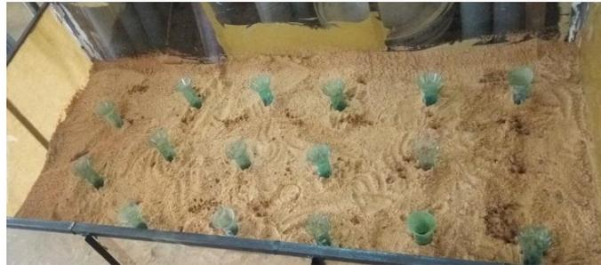
**Figure 6: Grid of rain gauges on the plot**
