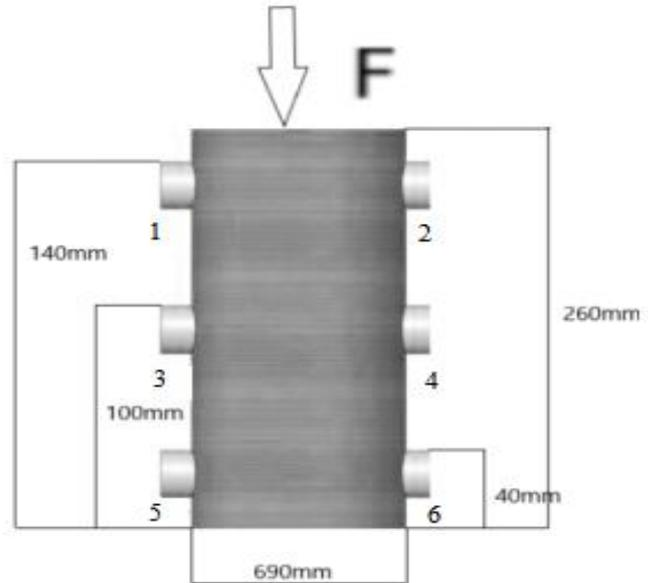
**Fig 4: Position diagram of acoustic emission sensors**
