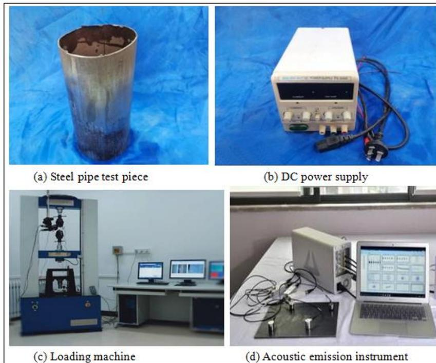
**Fig 1: Test materials and equipment**
