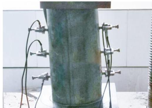
**Fig 6: Steel pipe pre-loading**
