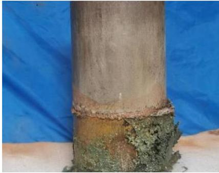
**Fig 3: Corroded steel pipe**
