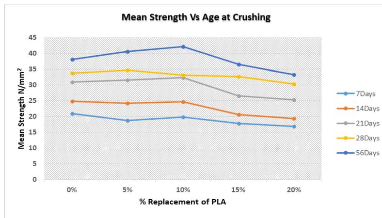
**Figure 1: Graph of Mean Strength Result against Percentage Replacement**
