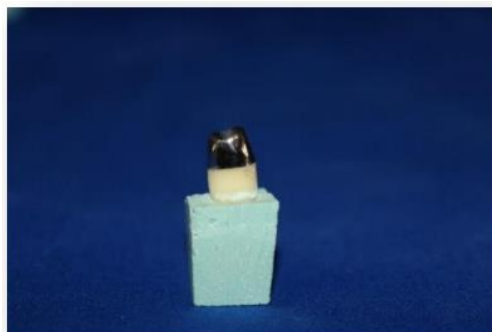
Fig. 1: Coping fabricated by Conventional lost wax method
