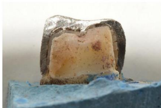
Fig. 7: Microleakage observed in Conventional coping
