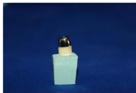
Fig. 2: Coping fabricated by direct metal laser sintering
