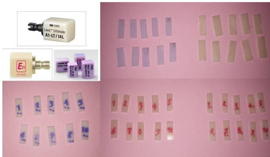
**Fig-1: Samples prepared from Lava Ultimate, IPS e.max CAD and Vita Enamic blocks**
