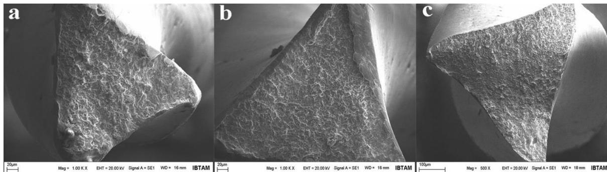
**Fig 2: SEM images of the One Shape instruments subjected to fatigue tests in interrupted rotation (a= One Shape 25.06, b= One Shape Apical 1, c= One Shape Apical 2).**
