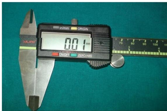
**Fig-1: Digital vernier caliper**
