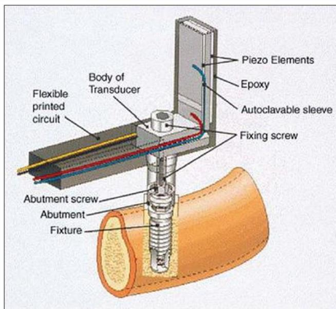
**Fig-1: Electronic Resonance Frequency Analysis**
