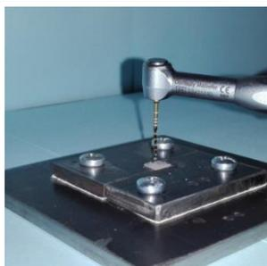
**Fig-6: Using X-Smart plus Motor (300 rpm, 2.0 Ncm) to rotate the file until failure occur**
