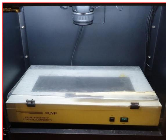
Figure 2. UV lamp apparatus set up
