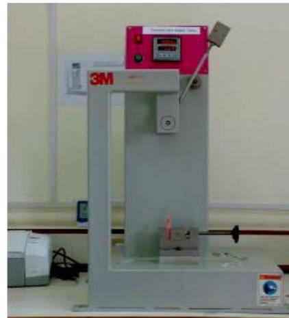
**Fig-7 :\_Notched IZOD Impact Tester**
