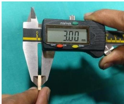
**Fig-7: Verifying the sample thickness**
