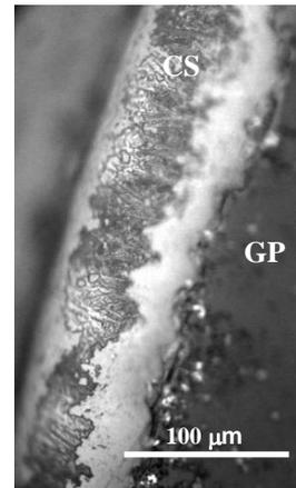
**Fig-3.** Layer of dendritic crystals developed on the surface of the sample 6B4Li, observed with Nital 2 attack.
