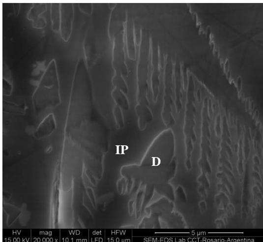
**Fig-4.** Crystalline layer in the PC sample in which dendrites (D) and interdendritic phase (IP) are observed.
