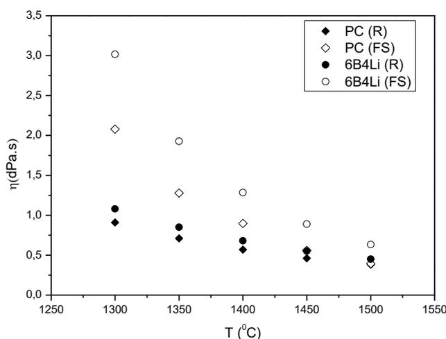
**Fig-1: Comparison between viscosity values obtained applying Fact Sage and Riboud model for PC and 6B4Li samples.**
