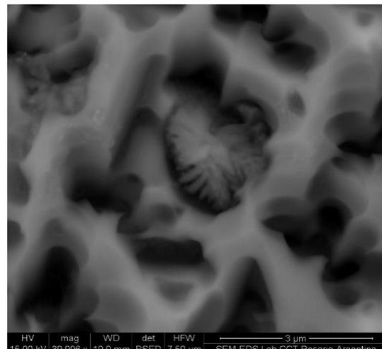
**Fig- 5.** Detail of the dendrite and interdendritic phase in the 6B4Li sample in the crystal layer.
