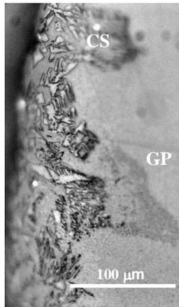
**Fig-2.** Layer of dendritic crystals developed on the surface of the sample PC, observed with Nital 2 attack.
