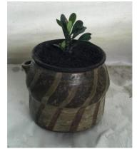
Fig-18: Planter 3 with the vitrified body as the reservoir (Body C)
