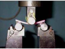
Fig-6: Three point bend test
