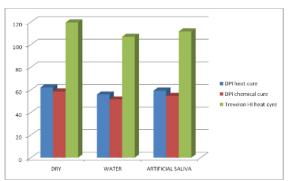
Fig-9: Graph depicting mean Flexural strength in different mediums
