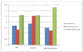
Fig-8: Graph depicting mean Impact strength in different mediums
