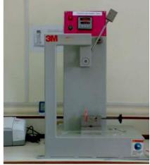
Fig-7 : Notched IZOD Impact Tester
